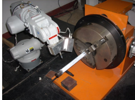
Figure 4: Calibration of positioner and robot
