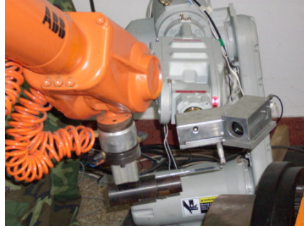
Figure 3: The calibration of two robots
