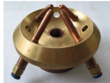
Figure 2 A novel conventional coaxial powder feeding head
