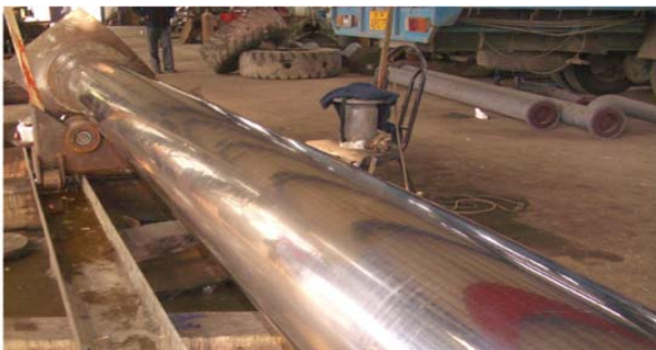
(Figure 8)The effect picture of restored hydraulic cylinder piston rod
