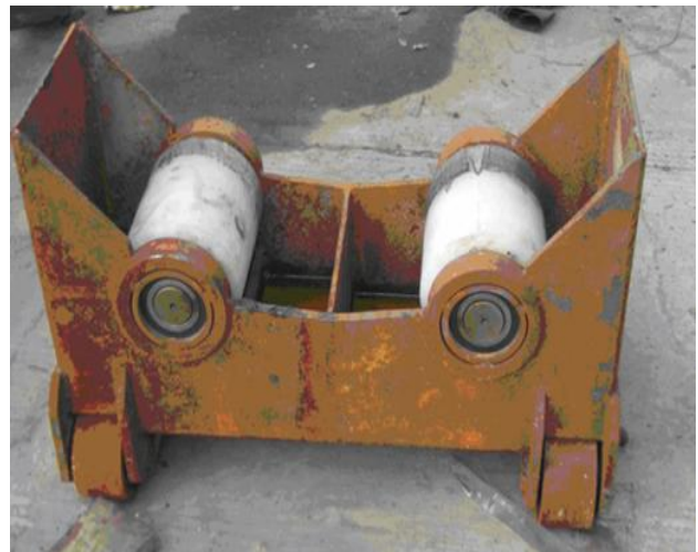
(Figure 4)Put 2 walking cars on the channel steel
