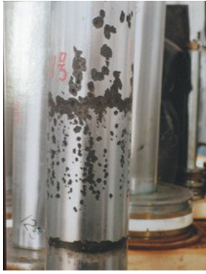
Fig. 2 (a) Worn and Corroded surface of the cylinder rod before maintenance
