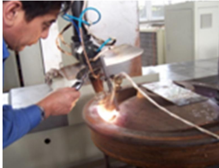
Fig.9: Laser remanufacturing lorry wheel.
