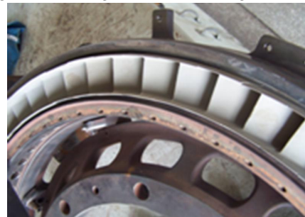
Fig.7: The first grade lamina after laser remanufacturing.
