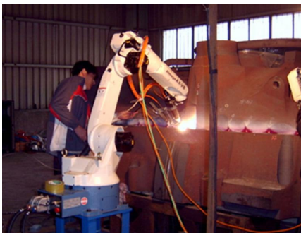
Fig.5: Field remanufacturing cylinder body of steamer turbine.
