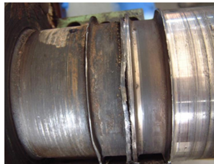
Fig.3: Conditions of atmosphere bearing location before laser remanufacturing.
