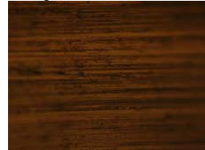
Figure 1 Surface topography after electrolytic degreasing at 14 volt
