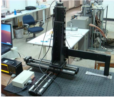
Fig.2 nonferromagnetic 3D electric controlled moving platform
