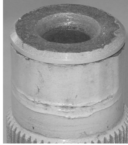
Fig. 1: worn torsion shaft
