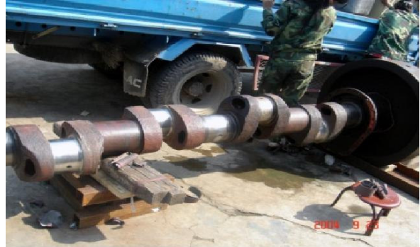
Repairing of crank shaft neck abrasion by electric brush
