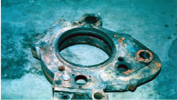
Repairing of casting blow hole and sand hole by casting disfigurement repairing machine
