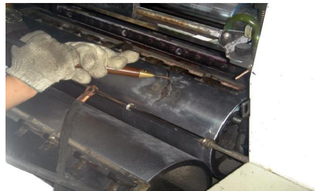
Repairing of the accessory by composite technics of resistance fusing welding and electric brush
