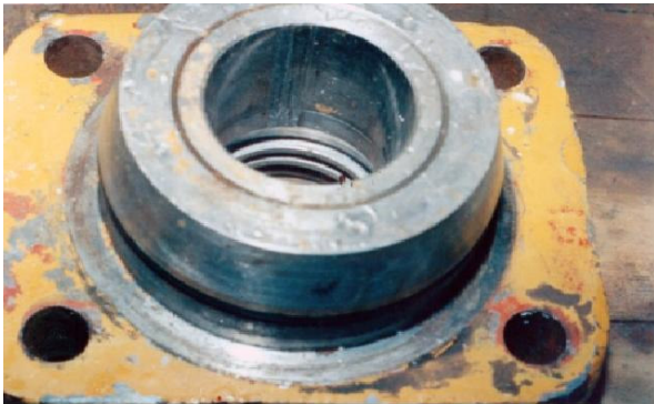
Repairing of casting blow hole and sand hole by casting disfigurement repairing machine
