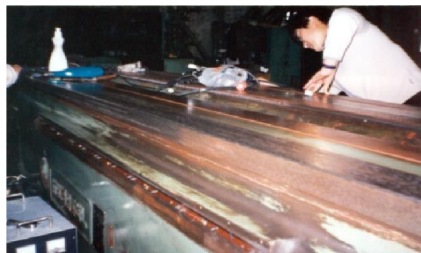
Repairing of machine tool guide rail abrasion by electric brush
