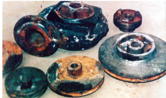
Repairing of casting disfigurement by adhesive
