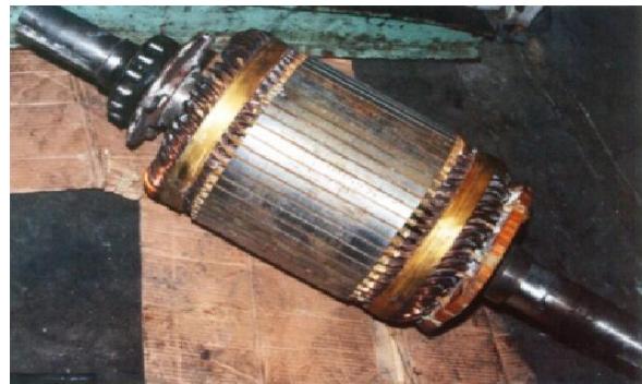
Repairing of mating faces of engine rotor axle tree abrasion by electric brush
