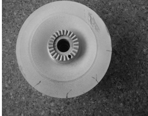
Fig 2 impeller crack show
