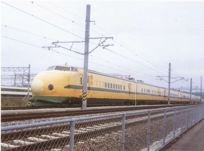
Shinkansen electric track total test train consisting of 7 cars (The RIVERNEW system installed on the 5th car)
