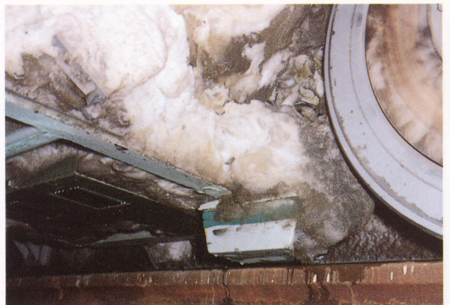
Status when optical type detecting equipment cannot be used because it is covered with snow (left side) and eddy-current sensor which functions normally even if covered with snow.
