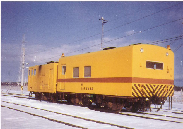
JR Track Inspector (RFD car) for JR Tohoku Shinkansen
