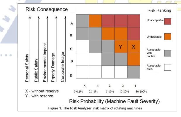
One of the most important tasks of the project was the development of Risk Analyzer software, what can classify the risk of rotating machines, which is under offline or on-line surveillance by diagnostic systems. The next figure 1 shows the risk matrix with the probability and the consequence variables.
