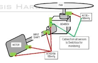
For maximum coverage, 6 sensors would be used on both the motor and gearbox for total of 12 sensors per installation. General purpose sensors like CTC's AC102 and AC104 series sensors rated at 100 mV/g would be recommended for applications
