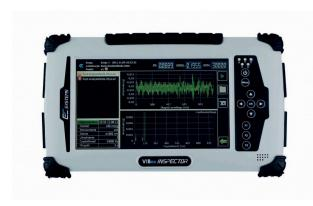
The AVM 1000DC/P is a single channel device recording vibration time signals together with machine's rotational speed registered on the second channel. Thanks to advanced vibration diagnostics methods the system detects in advance slowly developing machine failures like: bearings or gears damage, imbalance, misalignment and weak foundation. Early warning against failures makes it possible to replace the faulty elements before they cause further, greater damage to the machine.
