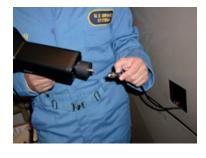
Adaptor Enabling Ultraprobe 15,000 To Read RAS Sensor.
