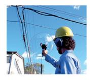
UWC-15: ULTRASONIC WAVE FORM CONCENTRATOR (PARABOLIC DISH) The UWC doubles the detection range of standard scanning modules and pinpoints ultrasonic leaks & electric emissions at great distances.
