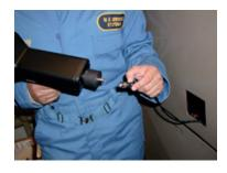
Adaptor Enabling Ultraprobe 10,000 To Read RAS Sensor
