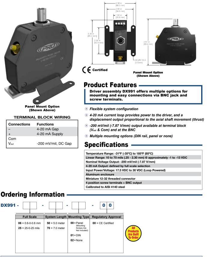
Example Part Number: DX991-25-70-01-00 4140 Steel, 25-0-25 mils full scale, 7 meter system length, DIN mount, CE certified
