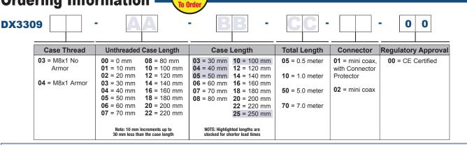
Example Part Number: DX330903-01-10-05-02-00 No armor, 10 mm unthreaded length, 100 mm case length, 0.5 meter total length, mini coax connector, CE certified
