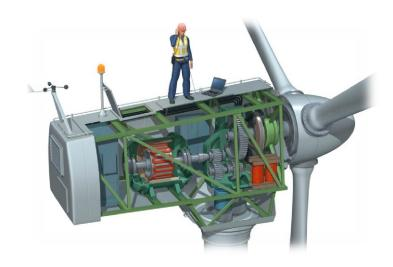
Using this web-based portal, Azima DLI provides regular status reports on all equipment and issues immediate alerts about serious faults. The WATCHMAN Remote service tracks and incorporates details such as widely varying wind turbine rotational speeds and in-line oil particle analysis into the monitoring system.
