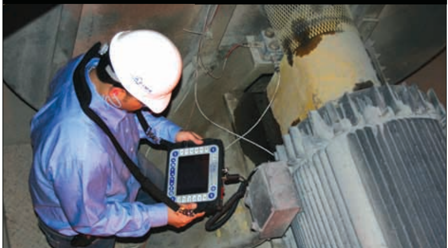
Figure 2. When a machine analyst collects vibration data from a forced draft fan at a 49 MW municipal waste combustion power generation plant in Haverhill, Massachusetts, it might be more cost-effective for that to be part of an outsourced machine condition monitoring program. (Azima DLI)
