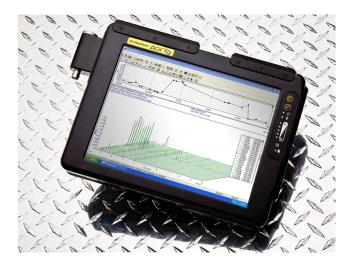
Azima DLI ALERT<sup>TM</sup> systems exist, machine data is automatically replicated through an innovative database technique that is transparent to the user. Whenever the mobile DCX unit is connected to the network by Wi-Fi or Ethernet, new data will automatically update all other DCX and networked ALERT systems. It's this functionality that makes competitive route-based data collectors obsolete.
