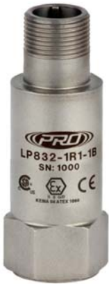
LP832-1B, Class I div 2 certified loop power 4-20 mA output-sensor,
