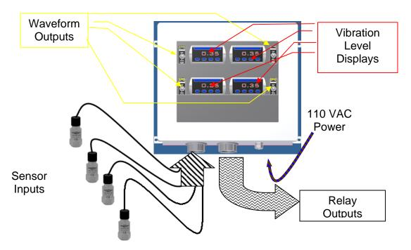
Figure 2. Cable Entry/Exit &Power
