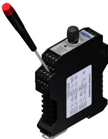
Figure 4. Terminal Block Removal
