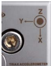
CTC sensor detail showing the orientation of the sensing elements
