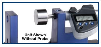
For increased accuracy, PRO has chosen to use a digital micrometer for measuring linear position. Multiple positioning holes for the probe mounts enables the linear field calibrator to be used with a large variety of probes. Current offerings include 5 mm and 8 mm probe mounts in both metric and English threading. Future offerings will include mounts for other probe sizes.
