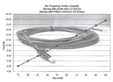
2. Temperature variability. While proximity probe are tested at more than one temperature, actual testing (when possible) in the ambient conditions (temperature/humidity) where the probes will actually be installed can provide the analyst with a more accurate baseline figure for dynamic measurements.
