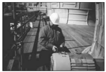
Figure 5 - Portable collection of vibration data from cooling tower motor.
