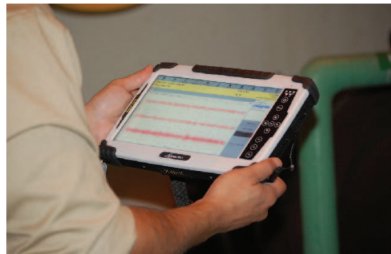
10.1" LED DISPLAY OFFERS A CLEAR VIEW OF MACHINERY DATA IN THE PLANT AND IN DIRECT SUNLIGHT.
