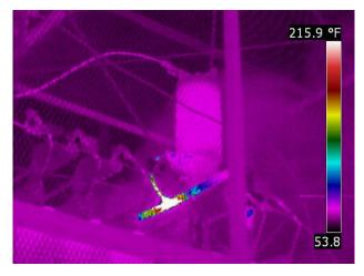
operating normally but the infrared inspection revealed a faulty wire connection and critical heat damage to the aluminum bus bar that would otherwise have gone undetected until failure.
