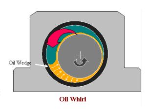
An oil whirl condition in a machine is serious and the unit should not be run except when absolutely necessary. The recommended repair and maintenance action is to inspect the turbine journal bearings. Specifically verify: proper bearing lubrication, proper bearing temperature and oil pressure, proper mechanical bearing fit in the housing and proper bearing clearances (tolerances) according to the bearing manufacturers specifications.
