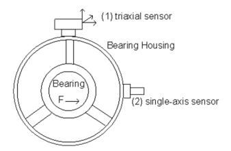
For measurement of machinery vibration for purposes of diagnostic trending, the difference in frequency response is usually not relevant. Both measurements are repeatable, so any increasing trend will still be detected.
