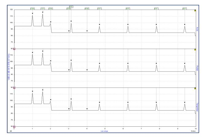
The baseline synthesizer requires only a minor amount of information from the user to accurately derive values for all amplitudes in 6 spectra per test location. This enables comparison of newly acquired data to the baseline for diagnostic purposes.
