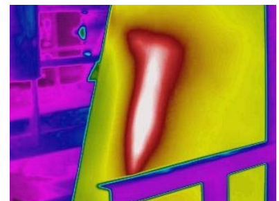
Vessel Refractory Failure
