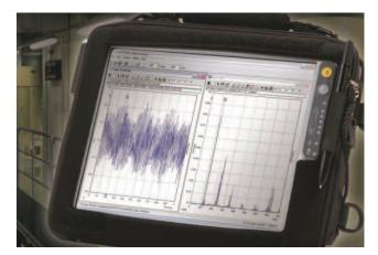
Using ExpertALERT's "User Defined Point" feature, special tests performed using RTA can be associated with machinery in your condition monitoring program and are accessible from the ExpertALERT tree. Click on the test and ALERT RTA (in viewer mode) will open up and display the appropriate data.
