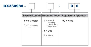
Example Part Number: DX330980-71-00 4140 Stainless Steel, 7 meter system length, DIN mount, no approvals
