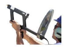
The UL101 and its attachments, like the PowerBeam 300, are utilized to extend the range of detection for pressure and vacuum leaks, electrical arcing and discharge, steam trap monitoring and more.
