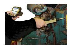
The UL101 and SoundCTRL is a powerful data acquisition and analysis system for condition based monitoring of critical equipment.
