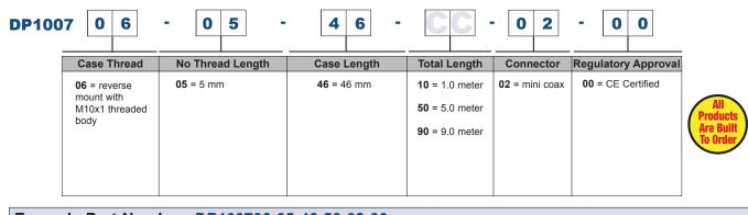
**Example Part Number:** DP100706-05-46-50-02-00 Reverse mount with M10x1 threaded body, 5 mm no thread length, 46 mm case length, 5.0 meter total length, mini coax connector, CE certified
