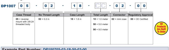
Example Part Number: DP100705-02-18-50-02-00 Reverse mount with 3/8-24 threaded body, 0.2 inch no thread length, 1.8 inch case length, 5.0 meter total length, mini coax connector, CE certified
