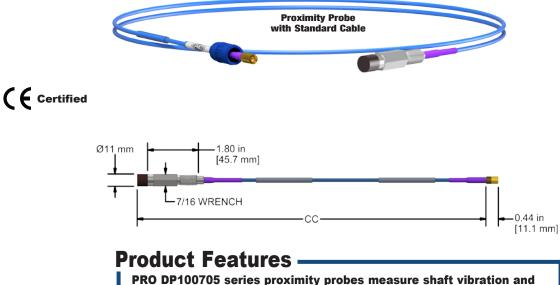
**PRO DP100705** series proximity probes measure shaft vibration and displacement on machinery with fluid film bearings. Durable **PPS** over-molded probe tips withstand harsh conditions when monitoring critical machinery such as turbines and compressors.
